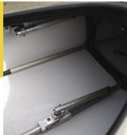
The hydraulics’ hand levers curve and lock to the aluminum frame members to avoid snagging. Small toggles on the aft end release the pressure to contract the piston.
